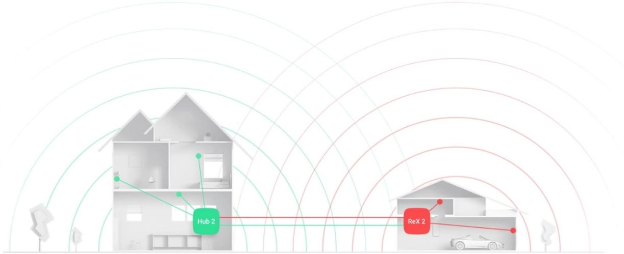
ReX 2 expands the radio communication range of the security system, allowing the installation of Ajax devices at a greater distance away from the hub.
